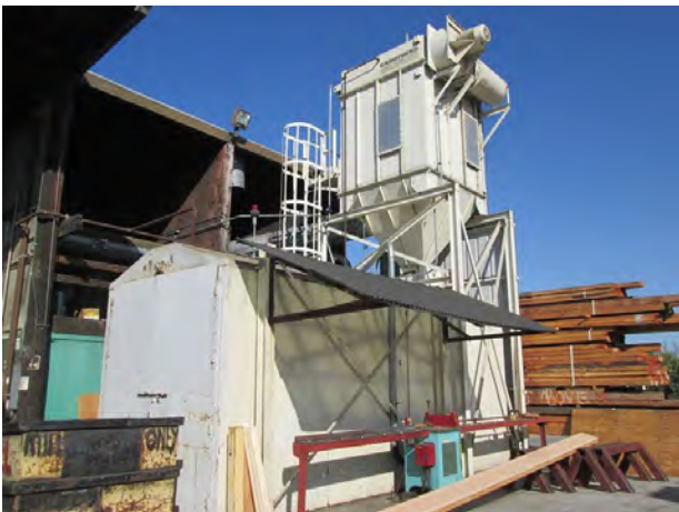
23. View of the dust collector for the main mill located on the northwestern portion of the subject property.
