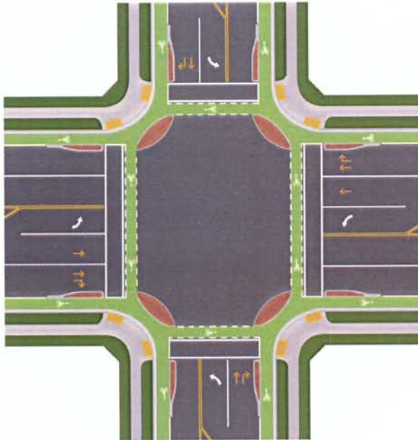
Figure 3-18 Protected Bicycle Lane Intersection
